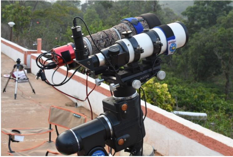
Astro Photography equipment with auto guider and cooled CCD monochrome camera and filters
