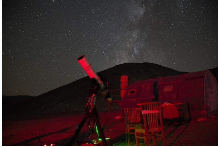
Astro Photography equipment with auto guider and cooled CCD monochrome camera and filters
